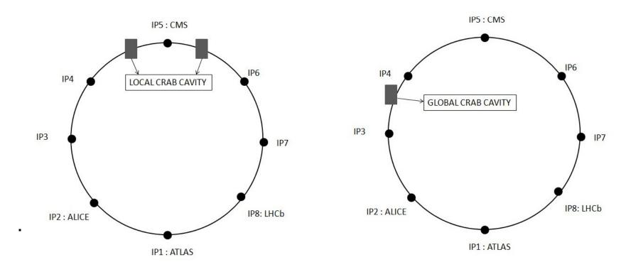
The simplest case is a single GCC. To simulate a crab-RF failure we vary the crab-RF voltage and the crab-RF phase.
