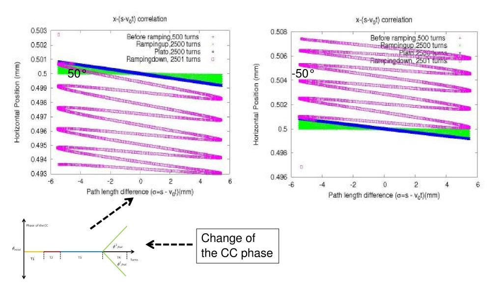
A CC phase change steers the beam at the IP as expected
