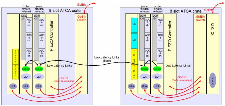
Piezo Controller configuration for ATCA LLRF:
