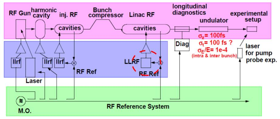
Accelerator subsystem must "play" together at the same time on order to achieve desirable acceleration of particle beam (beam energy and time parameters) and SASE
