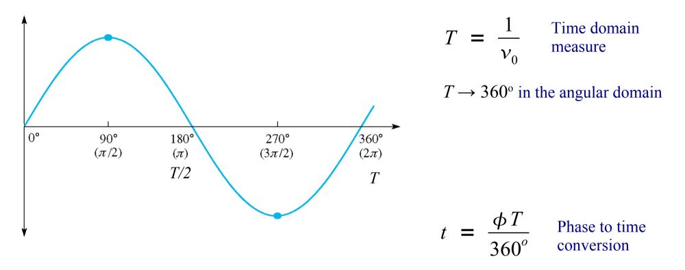
Example:  $v_0 = 1.3$ GHz  $\rightarrow T = \sim 769$ ps,  $1^\circ \rightarrow 2,13$  ps
