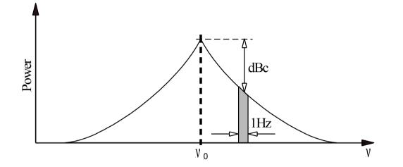
Power Spectral Density measured in dBc/Hz
