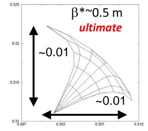
nominal tune footprint up to  $6\sigma$  with 4 IPs & nom. intensity  $N_b$ =1.15x10<sup>11</sup> L=10<sup>34</sup> cm<sup>-2</sup>s<sup>-1</sup> tune footprint up to  $6\sigma$  with nominal intensity and 2 IPs
