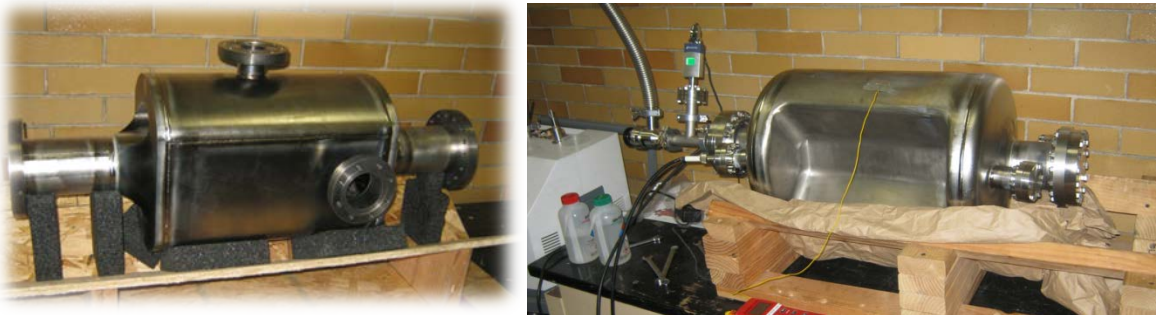
Figure: Prototype compact Nb-Ti crab cavities for the LHC: 4-rod cavity (left) and double-ridge cavity (right).
